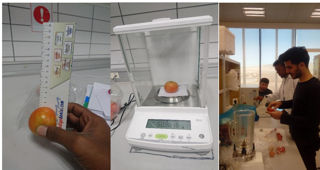
Figure: 3.7. (A); Measuring fruit width with ruler, (B); Weighting fruit(g) with digital weight scale, (C); Measuring soluble solid content (brix) by using A. KRÜSS Optronic GmbH, AR-2008.
