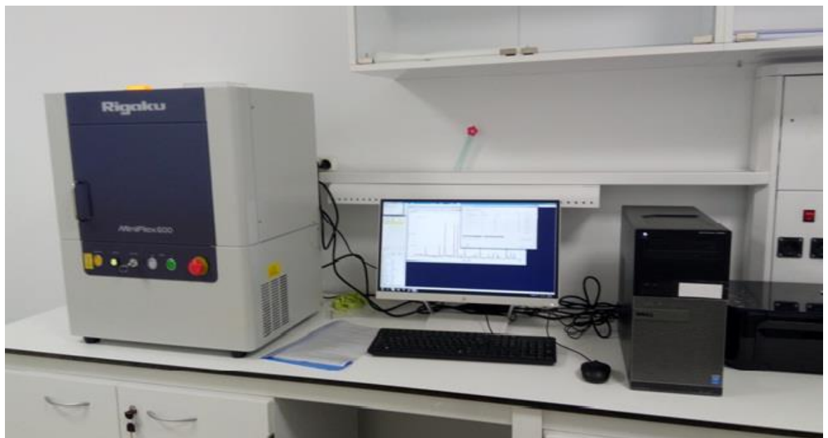
Figure 3. 12 XRD used in measurements
