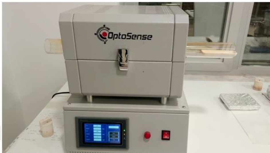
Figure 3. 4 OptoSense tube furnace used for annealing
