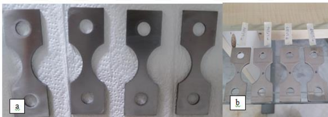
Figure 4.6 (a) Sanded and Ultrasonic Bathed Specimens (b) ID Numbered Specimens For 3.5 % Salinity Solution
