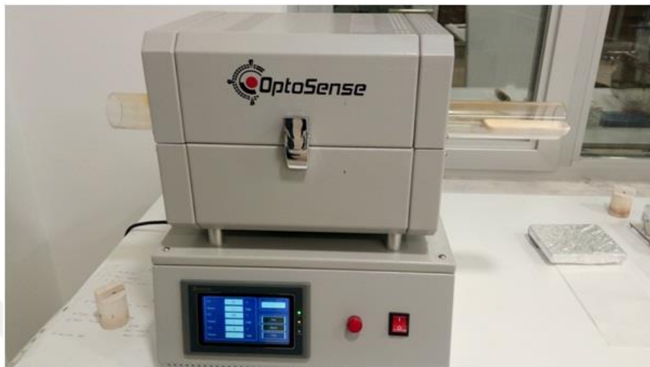
Figure 3. 4 OptoSense tube furnace used for annealing
