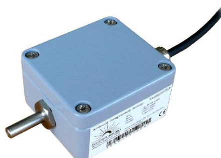
Figure 6.15 Ambient temperature sensor [80,81]
