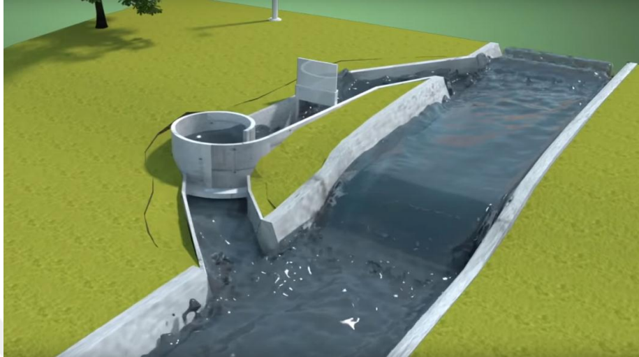
Figure 3.3 One of gravitational water vortex power station
