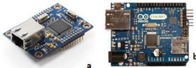
Figure 2.7 (a) Ethernet module that can be associated with any sensor; (b) Arduino board with installed Ethernet interface.
