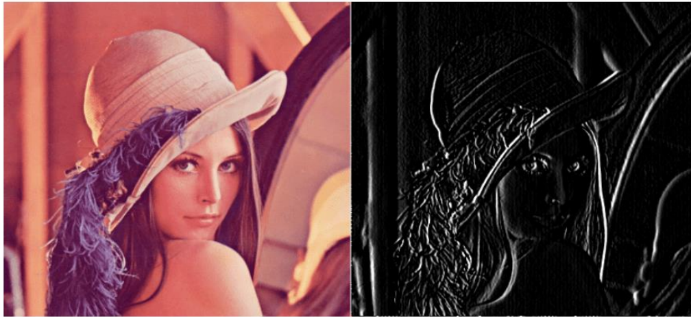
Figure 2.12 An image convolved with vertical Sobel filter
