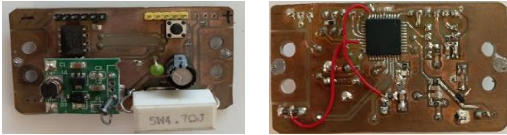
Figure 3.23 Real time implementation of designed Second BMS system slave controller card
