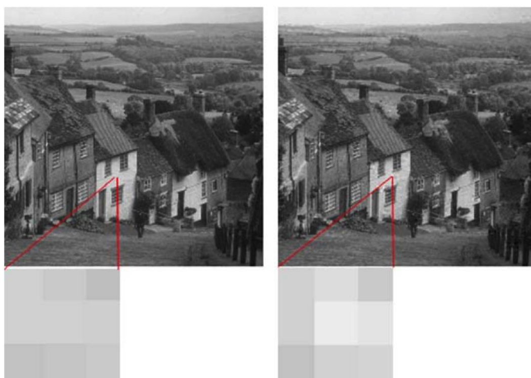
Figure 2.8 Embedding at the DCT level is quite unique and professional method as long as it is managed to be kept the artefacts at the out of the scope with carefully chosen coefficients. Otherwise, artefacts will be unavoidable as shown above.
