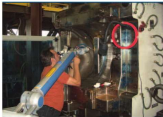
Mobile repair welding within the machine on a die-casting mould (Photo: Jutz Lasertechnik)
