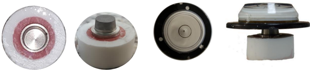
Figure 33. View of controlling the adequate positioning of each die in acrylic resin using bubble level tool
