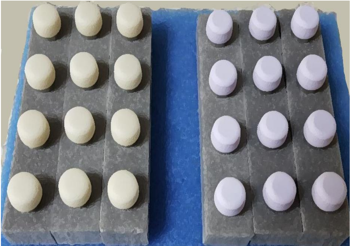
Figure 26. Pre and post sintering of Lithium disilicate crowns
