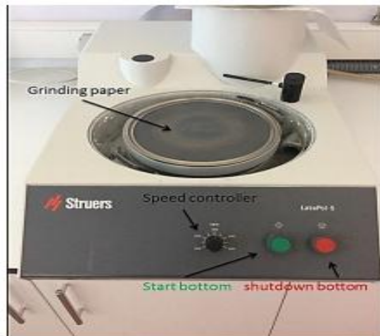
Figure 3.7. Grinding wheel rotating type machine.
