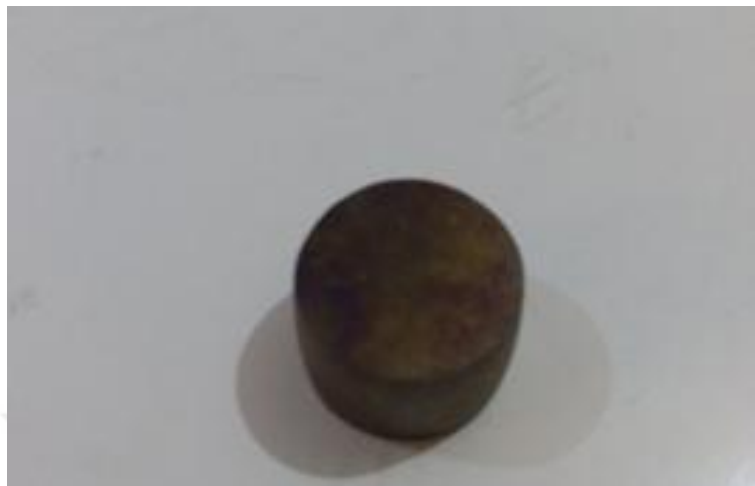
Figure 3.11. The macrograph of the sample sintered at 1200 °C for 1h without using Ti getters.
