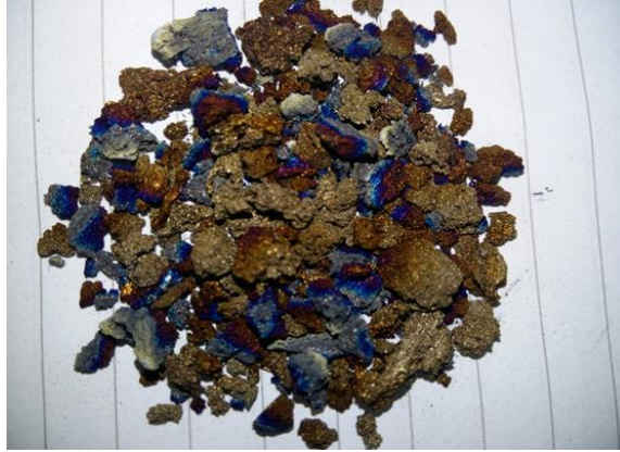
Figure 3.15. Oxidized Ti getters after high temperature (1200 °C) sintering process.
