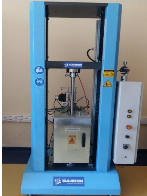
Figure 3.22. Uniaxial compression testing machine equipped with a heating-cooling system.
