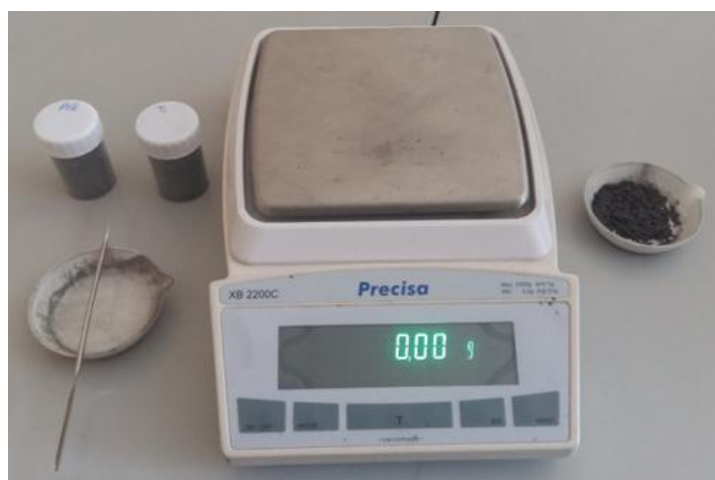
Figure 3.4. The electronic balance employed to measure weight of the raw powders.
