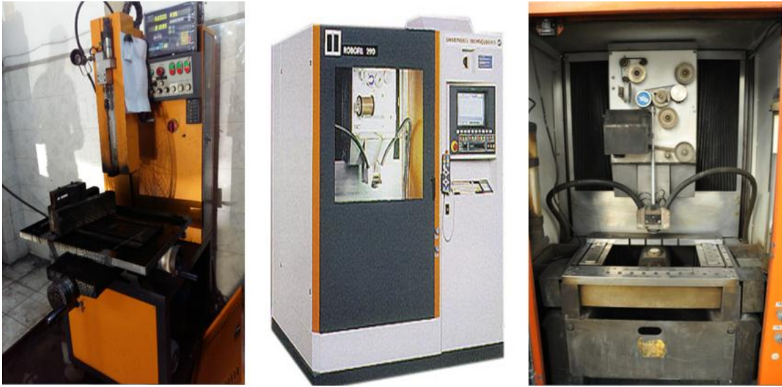
Figure 3.18 Two electrical discharge machines used for cutting samples.
