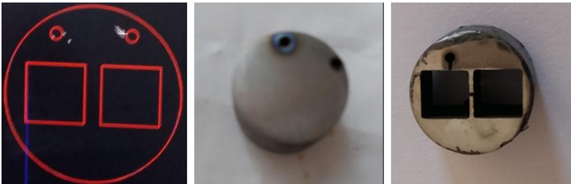
Figure 3.17. Processing of cutting samples with dimensions 5x5x10mm
