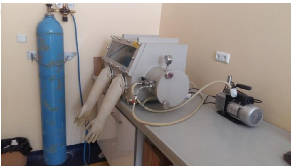
Figure 3.3 The argon-filled glove box used to store Ti and Nb powders.
