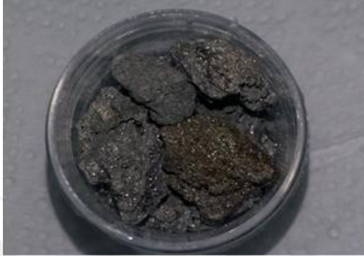
Figure 3.13. Ti sponge getters used during sintering.
