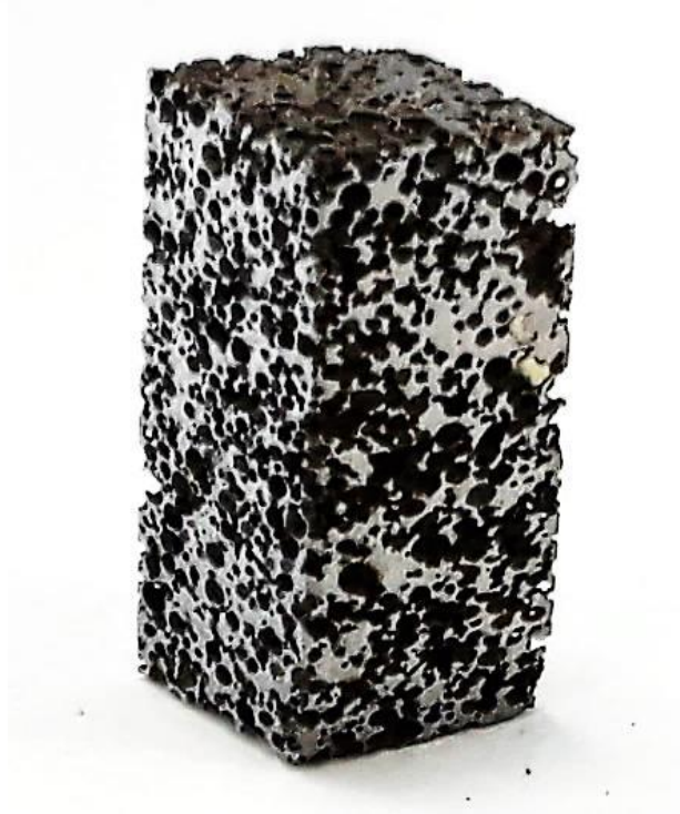
Figure 3.16. Ti_{74}Nb_{26} with 68% porosity sample after cutting by wire EDM with 5x5x10mm in dimension.
