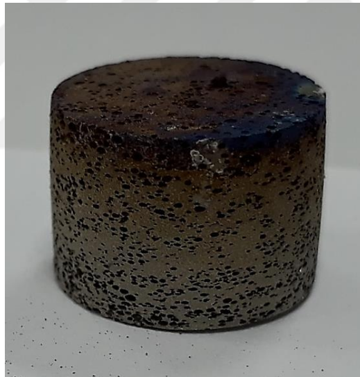
Figure 3.12. \text{Ti}_{74}\text{Nb}_{26} porous sample with 40% porosity cooled in the hot zone of the furnace after having been sintered for 4h at 1200^{\circ}\text{C} .
