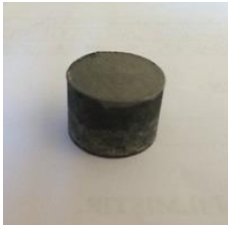
Figure 3.7. Sample hot pressed at 600°C under a pressure of 50MPa for 1h.
