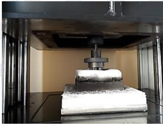
Figure 3.6. Powders in a graphite die under pressure inside the hot press furnace.
