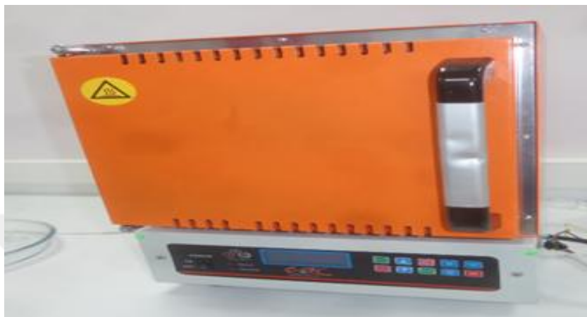
Figure 6. Furnace for calcination.
