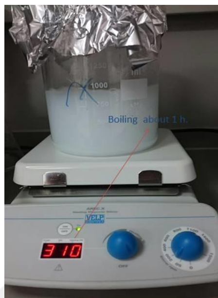
Figure 3.3. Shown the boiling the mixture from (130°C-310°C).
