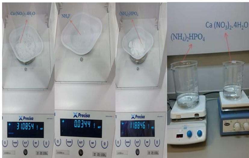
Figure 3.1. Magnetic stirring, to mixture each of the calcium nitrate tetra hydrate and di-ammonium hydrogen phosphate with pure water.
