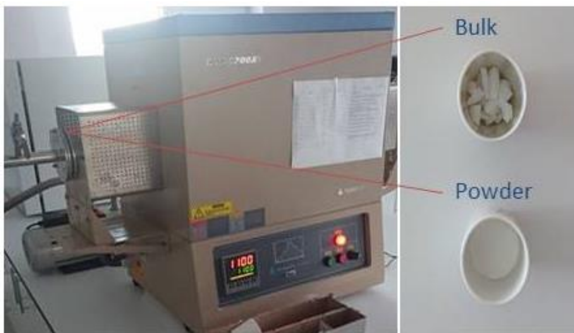
Figure 3.6. Shown the oven machine to sintering the mixture at 1100°C for 1 h.
