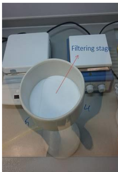
Figure 3.4. Shown the filtration of the mixture (TCP doped with ions).
