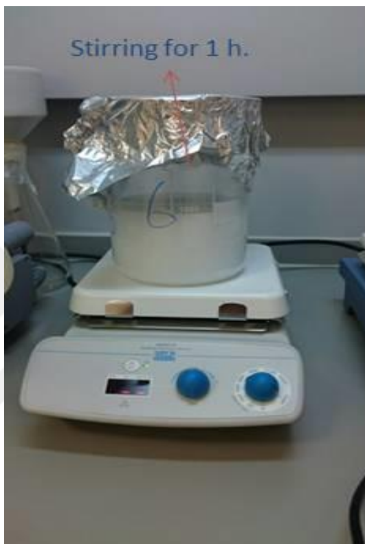
Figure 3.2. Shown the stirring and combine the TCP with ions.
