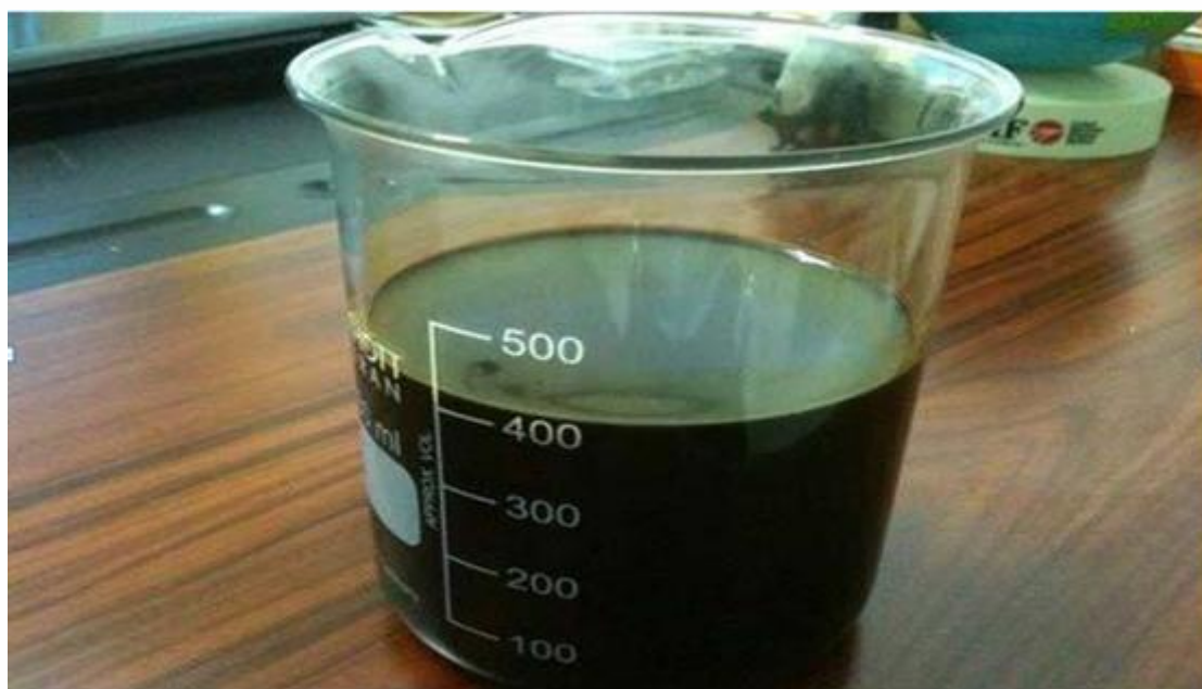
Figure 4.3. Sticky substance forming on the fuel sample after sulfur removal with formic acid.
