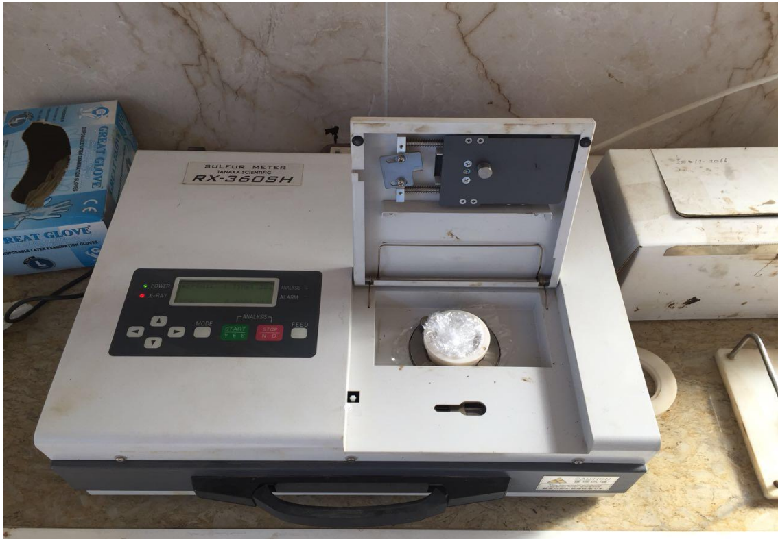
Figure 4.7. Measurement of sulfur in the fuel sample via sulfur measurement device.
