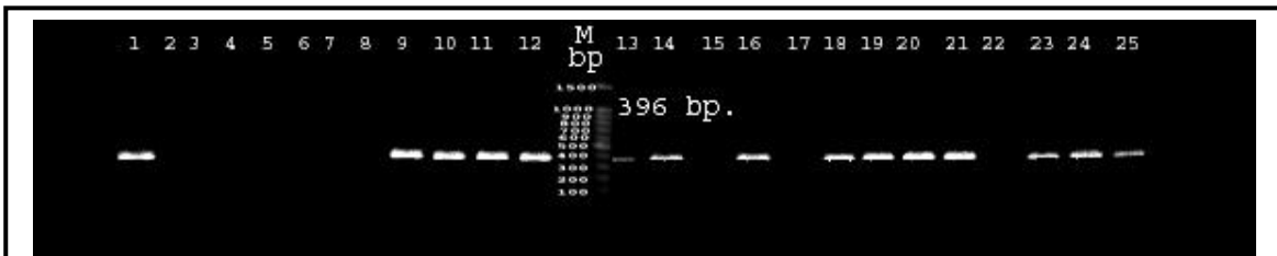
Figure 4.4. PCR amplification of P. aeruginosa isolates collected from Erbil area created toxA amplicon with molecular weight 396 bp. Electrophoresis was performed on 1% agarose gel and run with 5v/cm, for 1.30 hours. Path M contained DNA molecular weight marker (1500-100bp).
