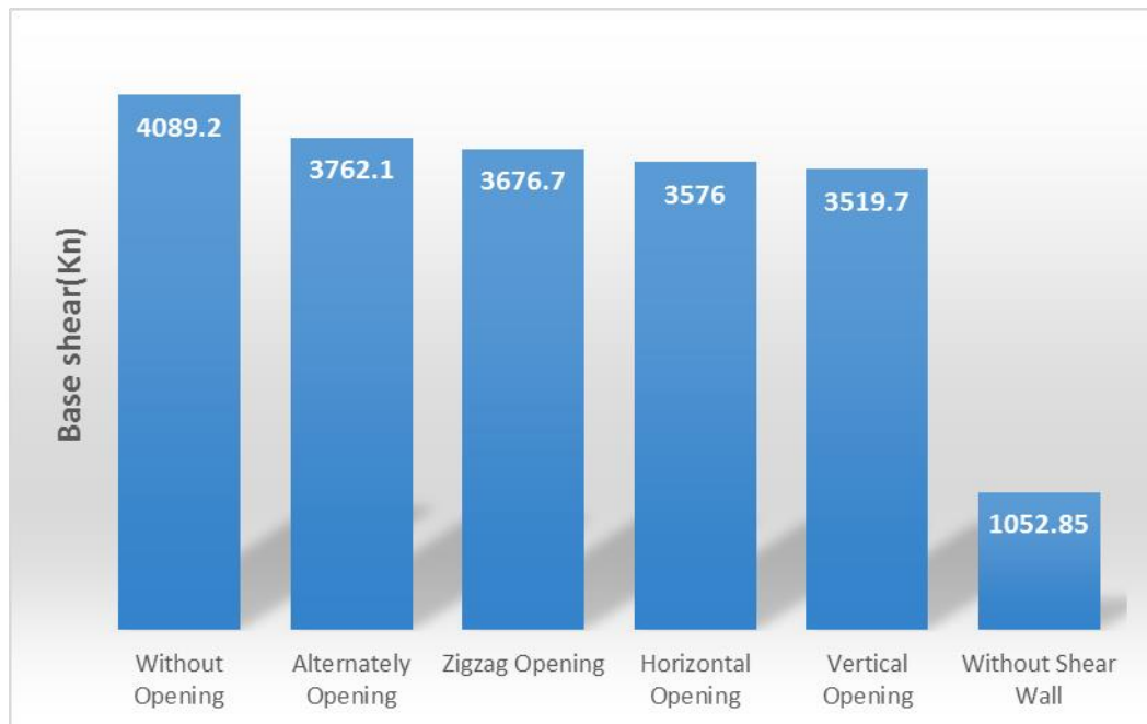
Figure 5.7. Shear base of the 5-stoty buildings based on the type of the shear walls.
