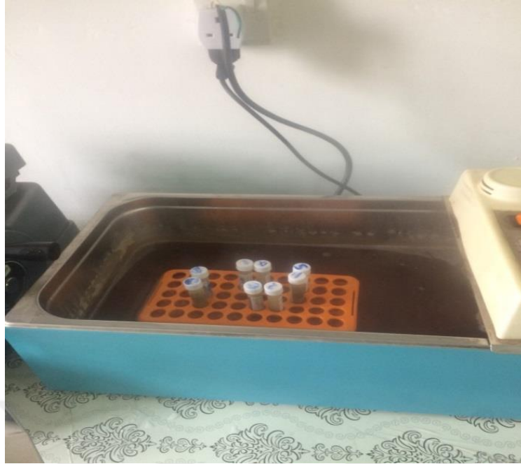
Figure 3.5. The samples in water bath (water bath temp: 90°C before the boiling point).
