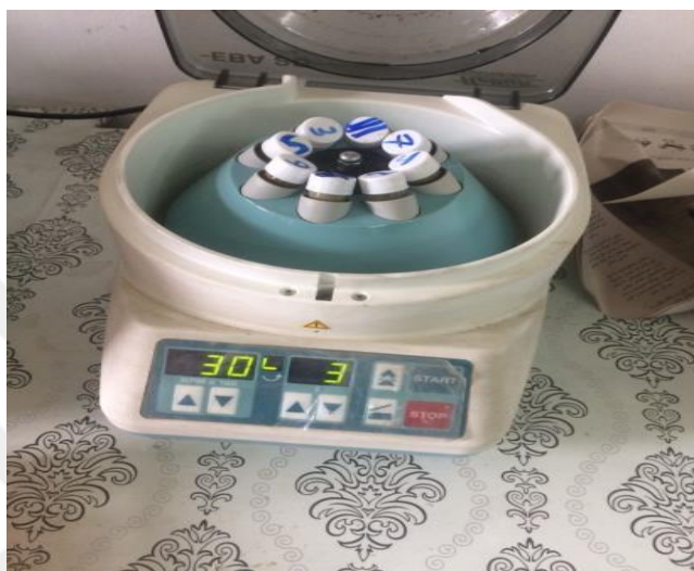
Figure 3.7. The samples in the centrifuge (speed: 3000 p.m. for PP test tubes).
