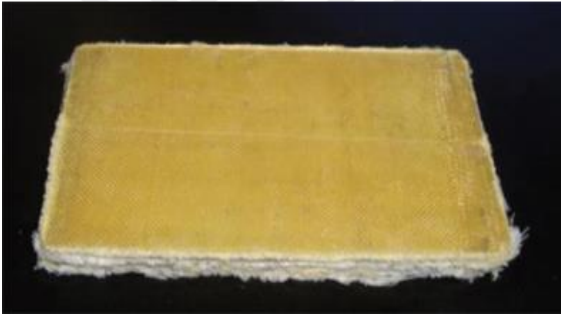
Figure 4. Final Kevlar29 - ramie composite (the front panel from the TSP).
