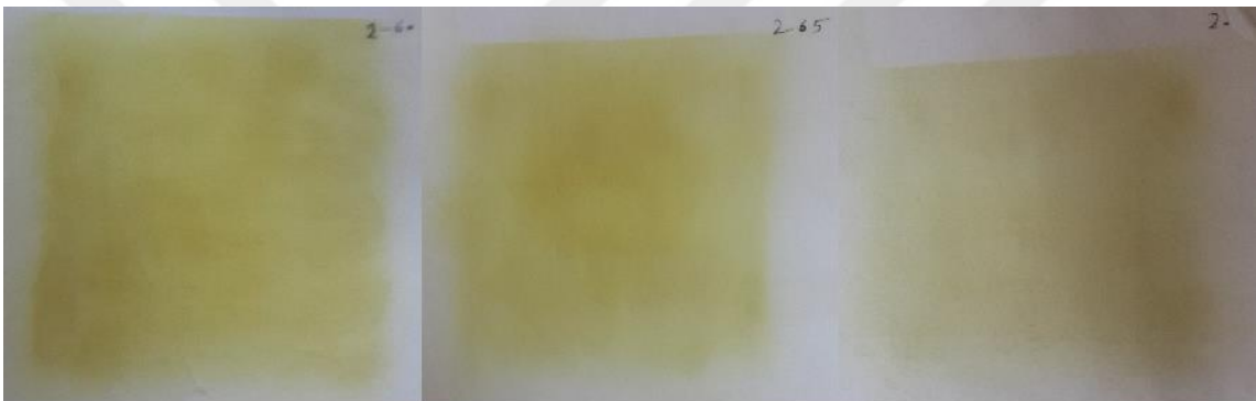
Figure 3.5. IR blocking sample with two layer graphene.
