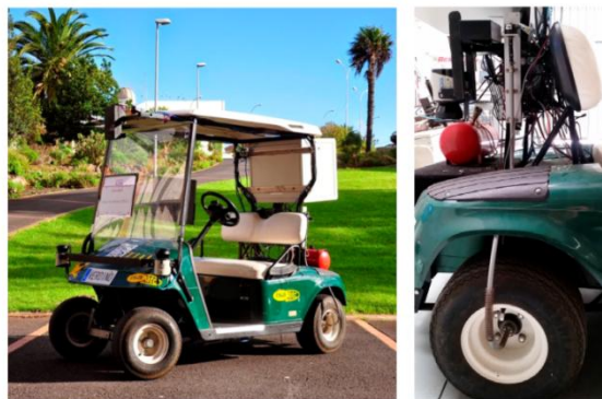
Figure 2.13. Shows the link between the odometric sensor and the encoder (Toledo et al., 2018).
