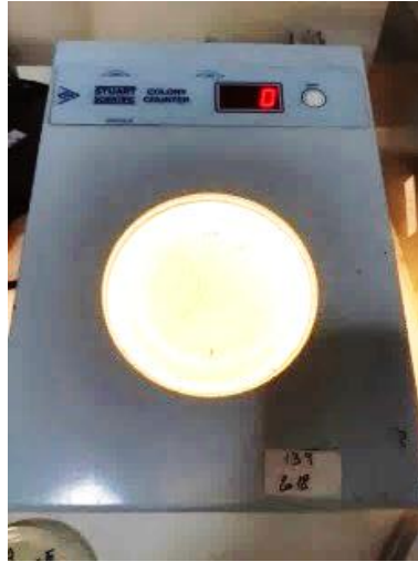
Figure 3.10. Colony counter stuart scientific SC5.
