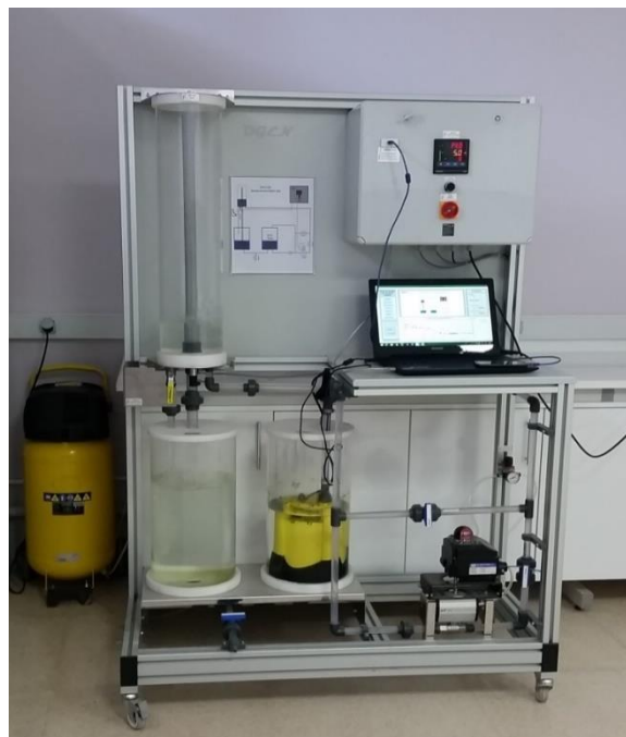
Figure 3.1 Experimental system: on-line computer connected liquid level control system.
