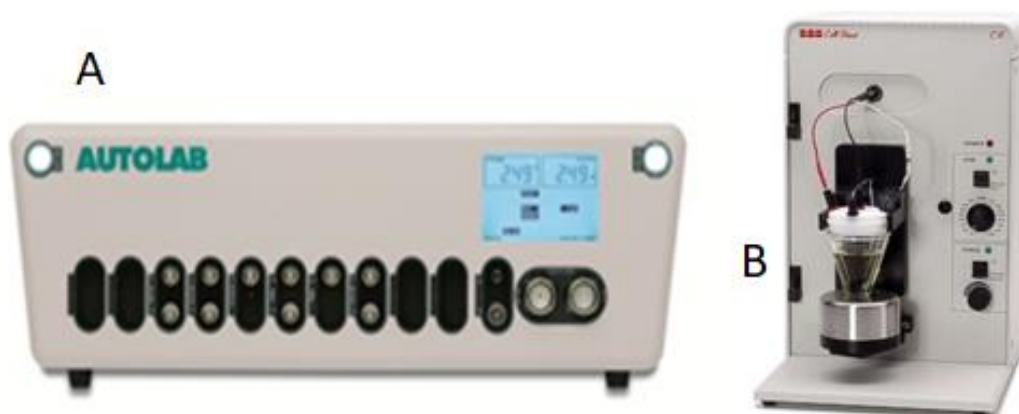
Figure 3.1. The electrochemical analyzer (A) and three electrode cell unit (B).
