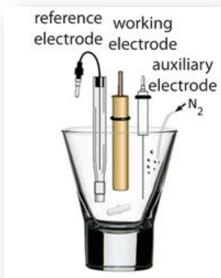
Figure 2.5. Electrochemical cell and its components (adaptation from Özkan et al., 2015).
