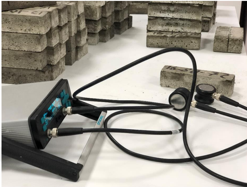
Figure 3.9. The ultrasonic pulse velocity test.
