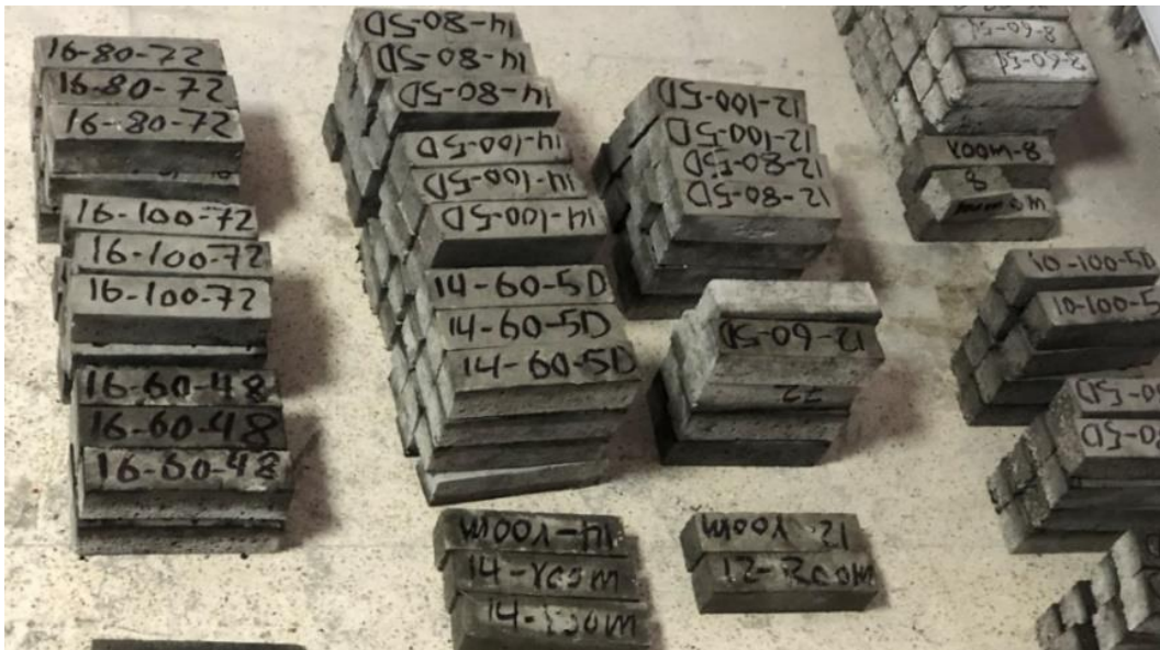
Figure 3.7. The specimens placed in room temperature until the testing time.
