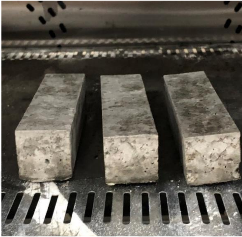
Figure 3.6. Curing the specimen in oven dry for different curing temperature and duration time.
