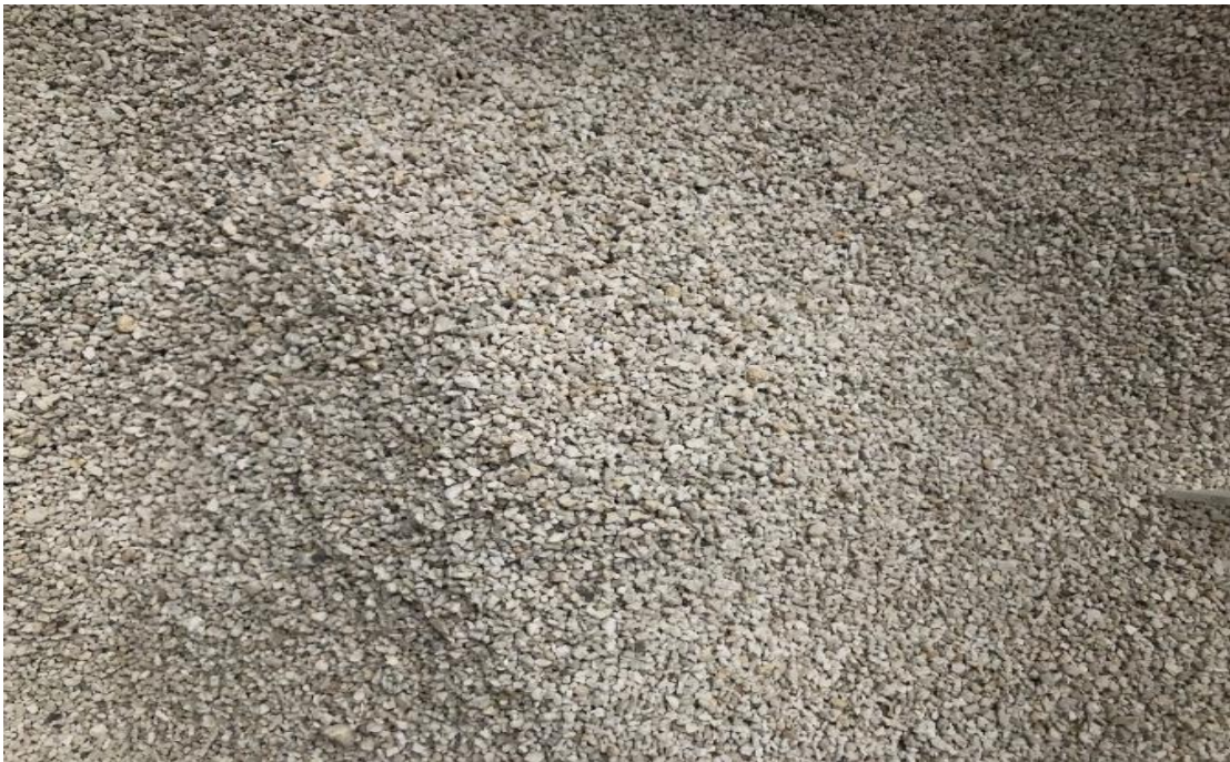
Figure 3.1. Pumice size aggregate between (0.5-3) mm.
