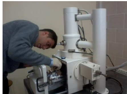
Resim 2.6. SEM-EDX Cihazı (Scanning Electron Microscope-Energy Dispersive X-ray)
