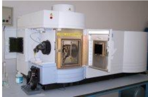
Resim 2.10. ICP-OES Cihazı (Inductively Coupled Plasma Techniques-Optical Emission Spectrometry) (Anonim, 2010).
