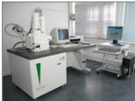
Resim 2.6. SEM-EDX Cihazı (Scanning Electron Microscope-Energy Dispersive X-ray)
