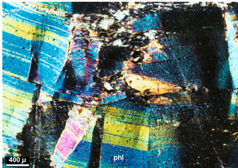
Figure 25. Photomicrograph showing kink banding in phl crystal from a PHLtite sample (analyzer in position).
