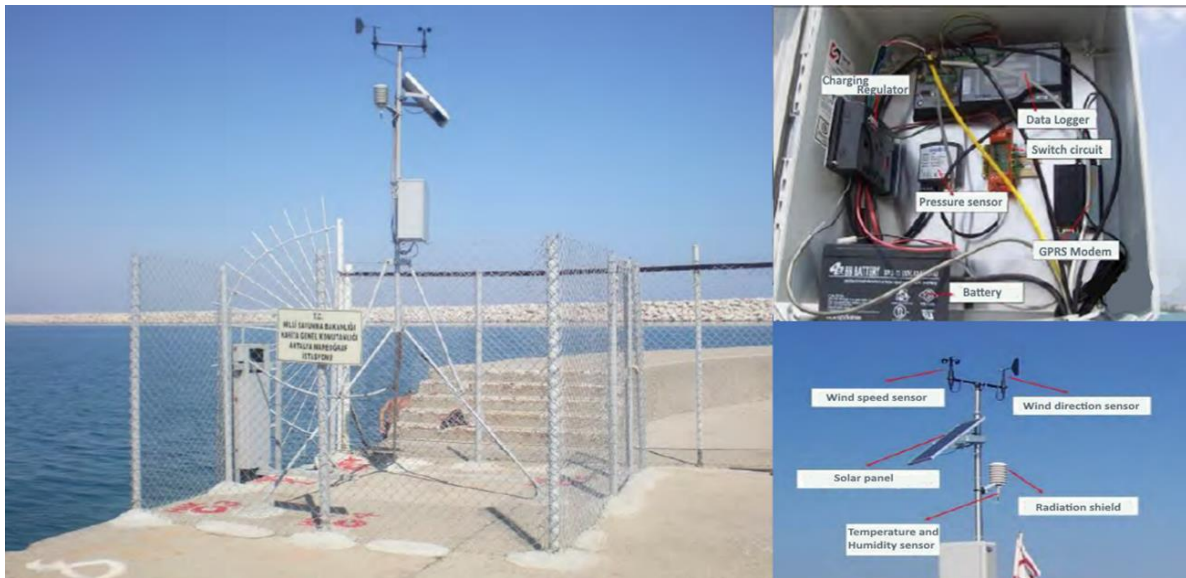
a) Digital and automatic acoustic-type tide-gauge (1998–2019) (left), the TUDES data transmission system (top-right), the integrated measurement systems for meteorological parameters (bottom-right).
