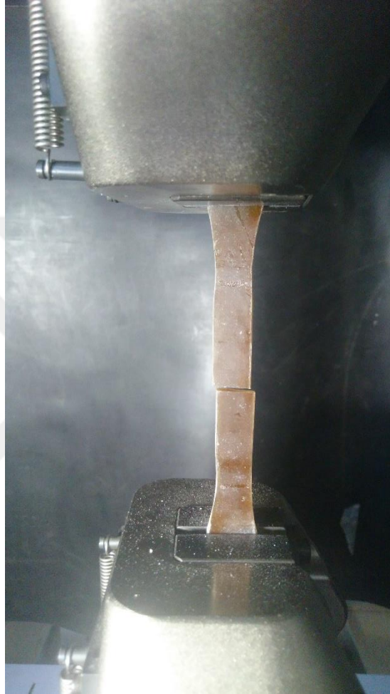
Figure 3.18. The specimen after the tensile loading
