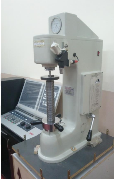
Figure 3.22. Hardness testing machine
