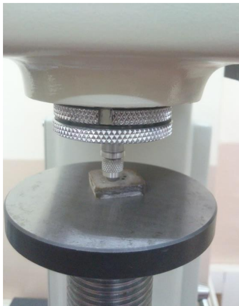
Figure 3.23. The specimen during the hardness test
