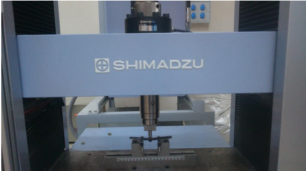
Figure 3.20. Flexural testing equipment
