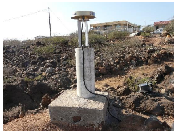
Figure 3.3. DJIG station (IGS) with Dorne Margolin and choke rings.
