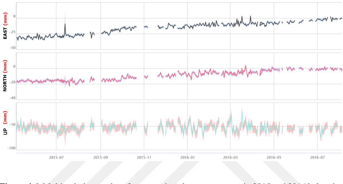
Figure 4.6. Multipath time-series of east, north and up components in 2015 and 2016 belonging to MAYG station.
