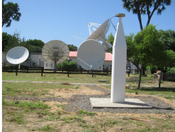
Figure 4.15. The presence of the reflective surfaces around the receiver of the MAL2 station.
