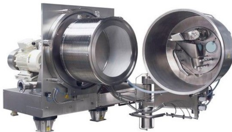
Figure 1.5. A filtering centrifuge with horizontal bowl for pharmaceutical applications. (Heinkel Drying and Separation Group, 2019)
