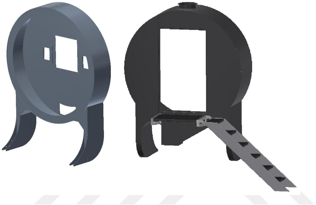
Figure 3.26 Material inlet & outlet section
