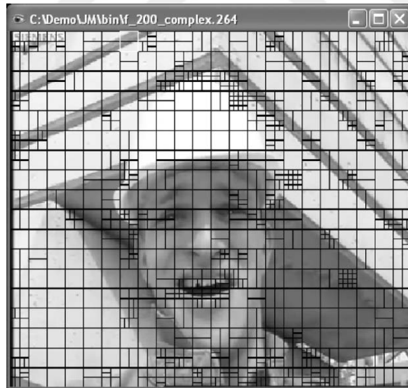
Figure 2.8. Example of partition choices for a P frame (Richardson and E. 2010)
