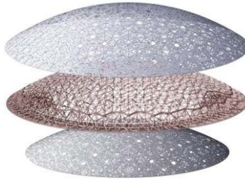
Şekil 4.41. Louvre Abu Dhabi, kubbe katmanları ( http://www.jeannouvel.com/en/projects/louvre-abou-dhabi-3/ , 2019)
