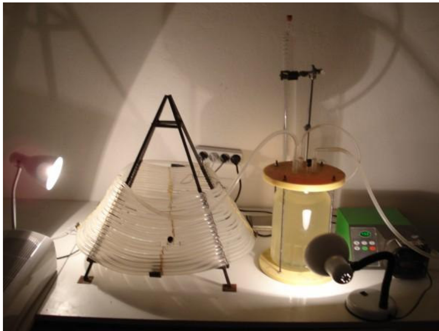
Figure 3.5. The recycling helical photobioreactor at start-up.
