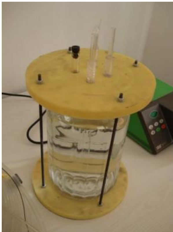
Figure 3.1. The 5-L reservoir and the fittings on the polyamide cover.
