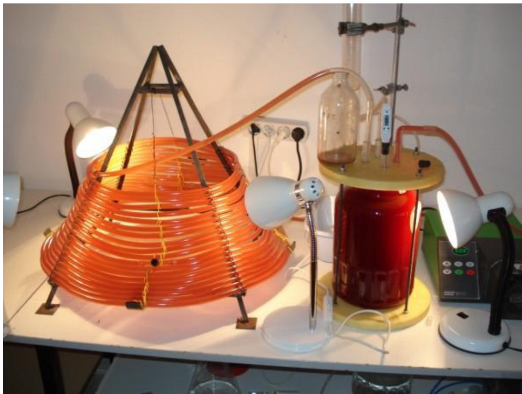
Figure 4.19. The recycling helical reactor in operation.
