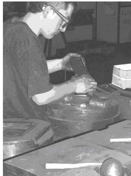
Figure 1.6 Manual polishing on die surface [8]
