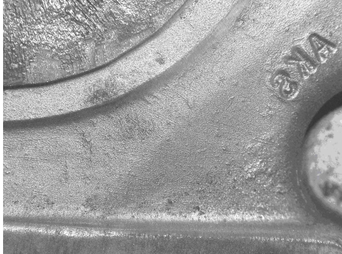
Figure 1.4 The surface manufactured by using EDM [8]
