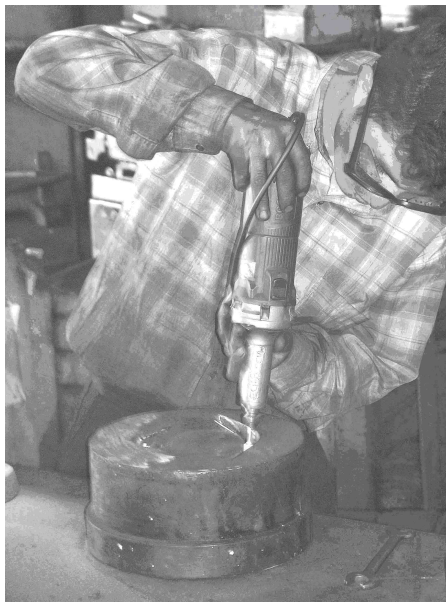
Figure 1.5 Manual polishing on die surface [8]
