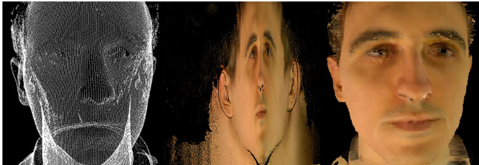
Figure 1.1 : a) 3D Face Model, b) Texture Image to Cover the Face, c) Texture Covered 3D Face Model
