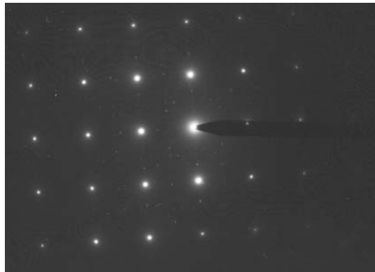
Fig. 4.12. SADP of the Al - 4 wt.% Cu alloy aged at 125^\circ C for 28 hrs.
