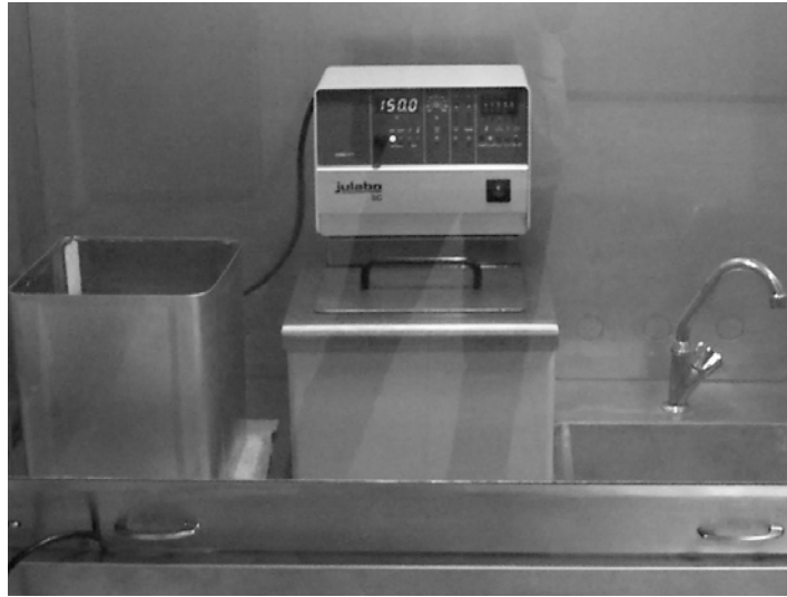
Fig. 3.5. The Julabo SC-12 oil bath, used for aging treatments.
