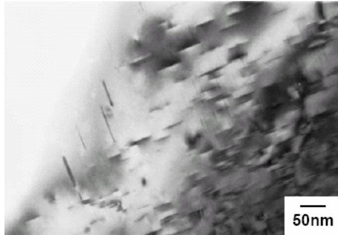
Fig. 4.14. Bright field image of the 10 vol.% B 4 C composite aged at 175°C for 8 hrs.
