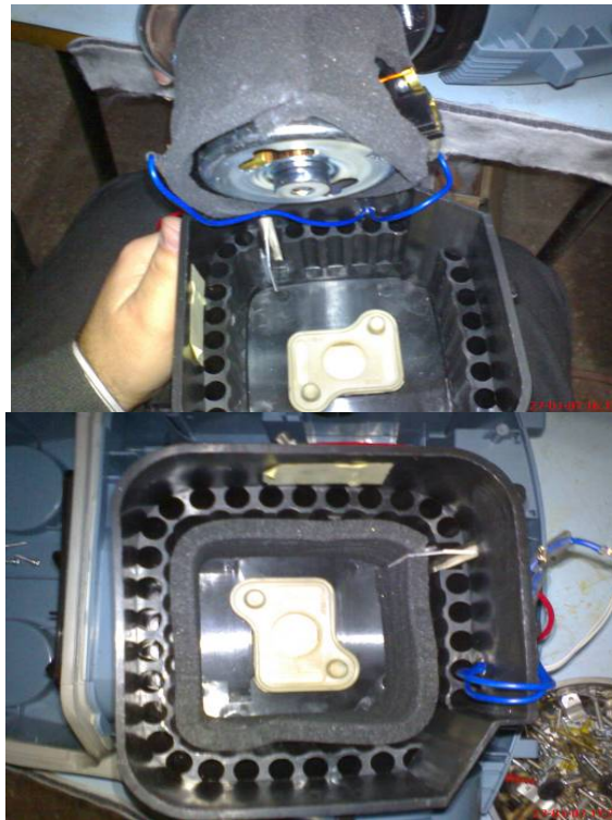
Figure 5.3.b Motor Casing without coating on the left; Motor Casing coated with the special black sponge on the right
