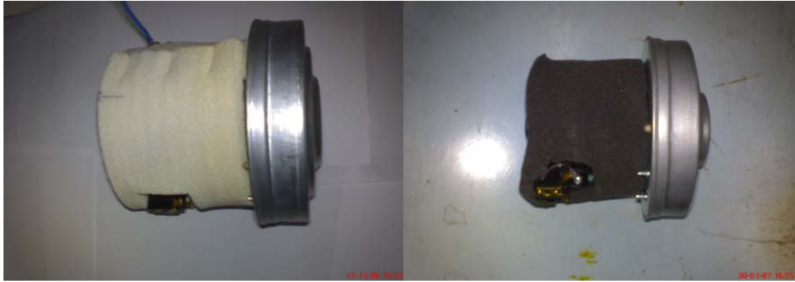
Figure D.5. Electric motor with Damping Material
