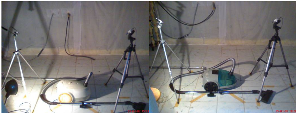
Figure 5.1. Prototype and Commercial Products in the Semi,-anechoic chamber
