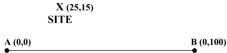
Figure 3.2: The closest distance of the site to the fault trace
