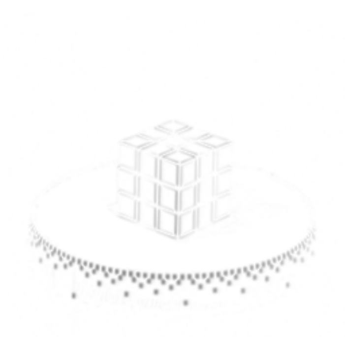
Figure 5.3: Output of the E_t gradient computation on FPGA hardware. The pixel values are inverted to get better visualization. White represents the lowest value and black represents the highest value.
