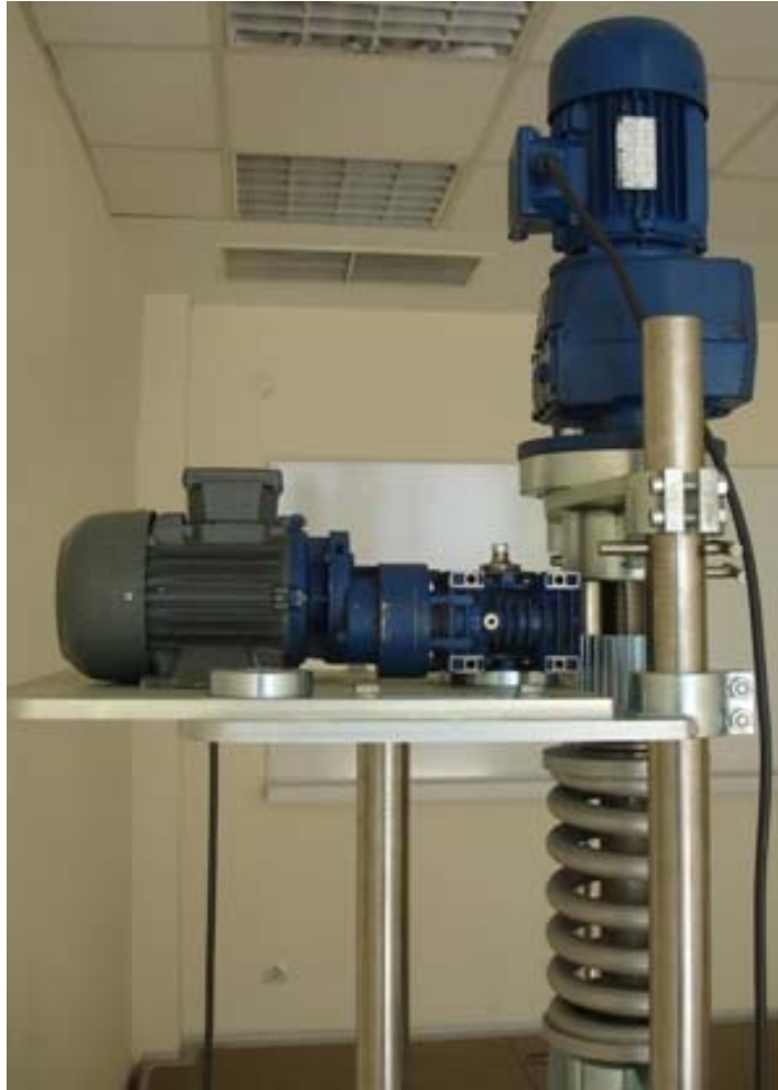
Figure 3.5 Photograph of reduction gear motors and the spring.
