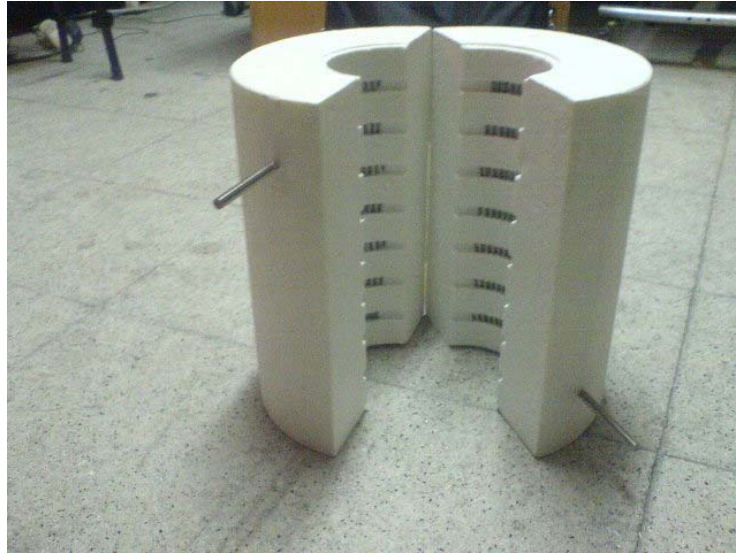
Figure 4.5 Furnace refractory elements with embedded Khantal resistors
