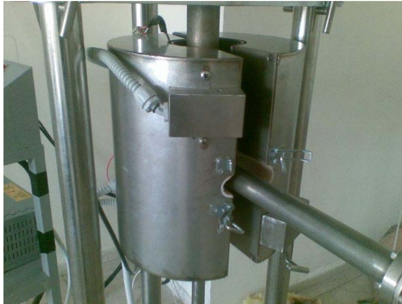
Figure 3.7 Split furnace used in the experiments
