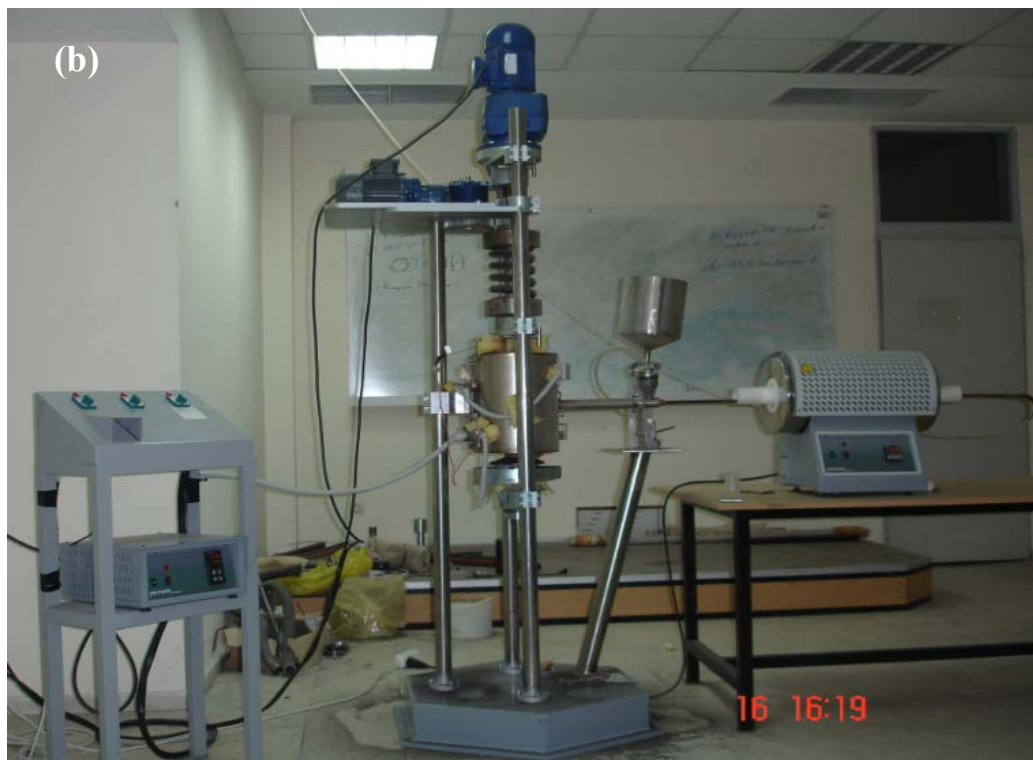
Figure 3.1 a) Schematic representation of test setup simulating operating condition of the thermal power plant boiler tubes b) Photograph of the test apparatus
