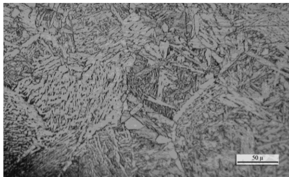
Figure 37 Microstructure of HAZ near the fusion line. The darker region on the lower left corner is the fusion line.
