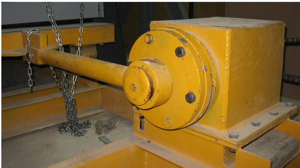
Figure 3.5. Rigid shaft and two attached discs
