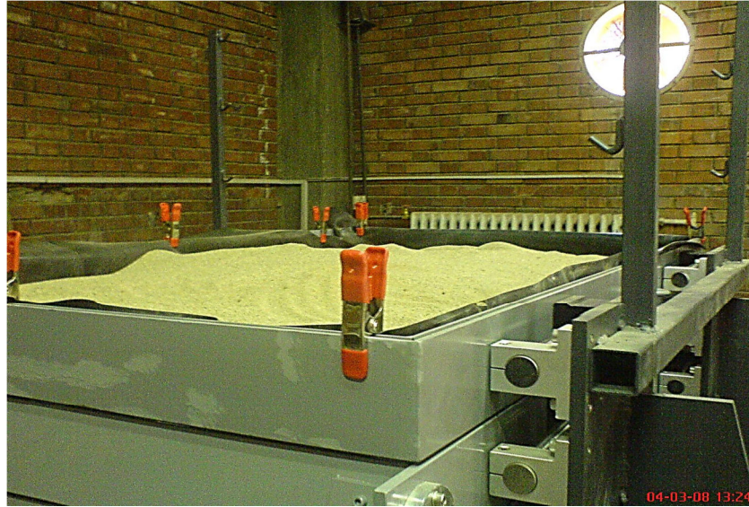
Figure 3.21 Laminar box after filling sand
