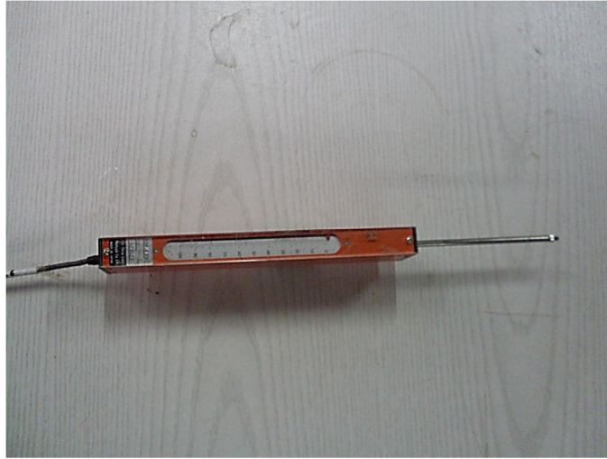
Figure 3.14. Displacement transducers used in shaking table tests.
