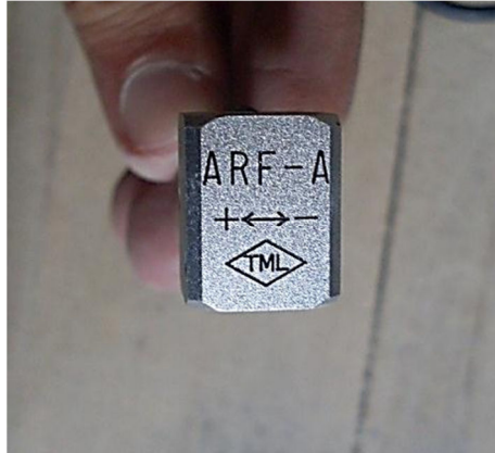
Figure 3.11. Acceleration transducer used in shaking table tests
