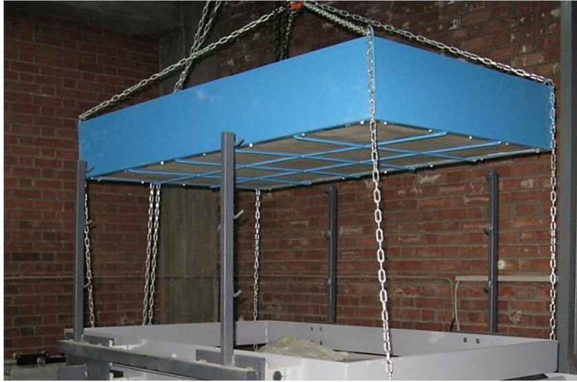
Figure 3.19. Diffuser with 2.36mm sieve size located on top of the laminar box
