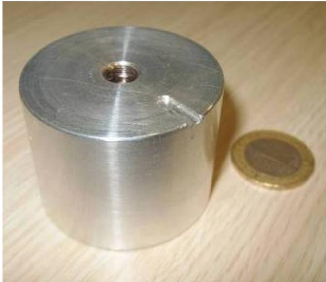
Figure C.15 Aluminum Apparatus for Modal Shaker Connection
