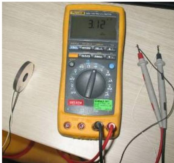
Figure C.3 NCE40 Capacitance Measurement
