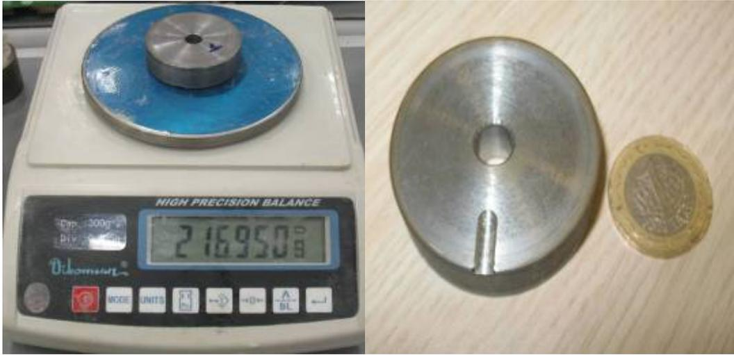
Figure C.14 Sample Steel Compression Mass in Harmonic Loading Tests
