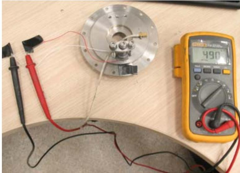
Figure C.6 CMAR04 Capacitance Measurement after Tightening for Pressure Gun Tests
