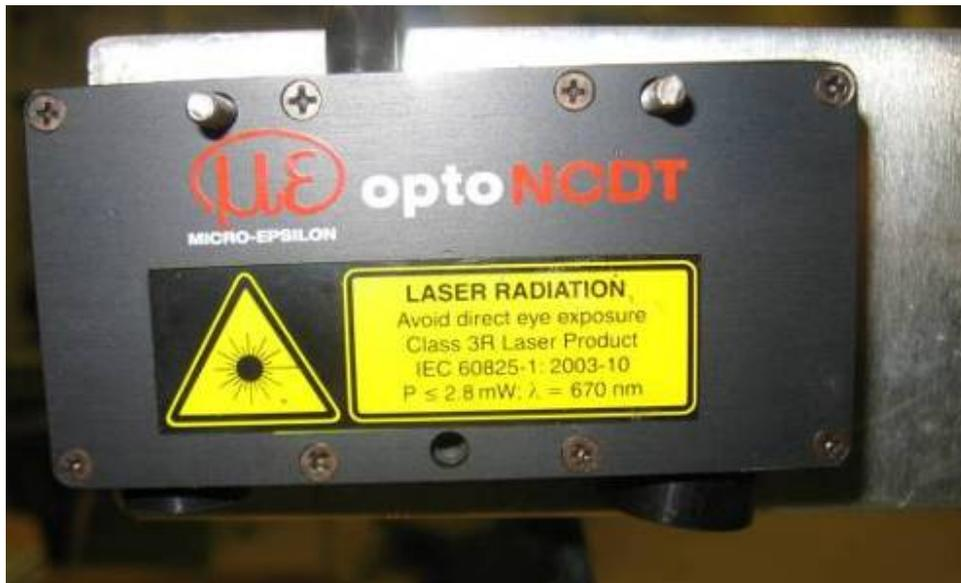
Figure C.19 Micro-Epsilon Laser Displacement Sensor
