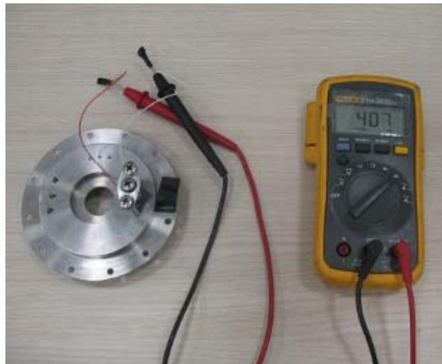
Figure C.5 CMAR03 Capacitance Measurement after Tightening for Pressure Gun Tests
