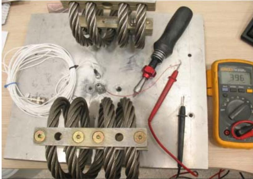
Figure C.4 CMAR03 Capacitance Measurement after Tightening for Impact Hammer Tests
