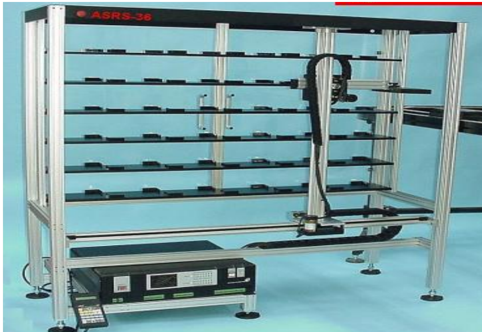
Figure 1. 2: Intelitek AS/RS: Physical System and Controller Unit
