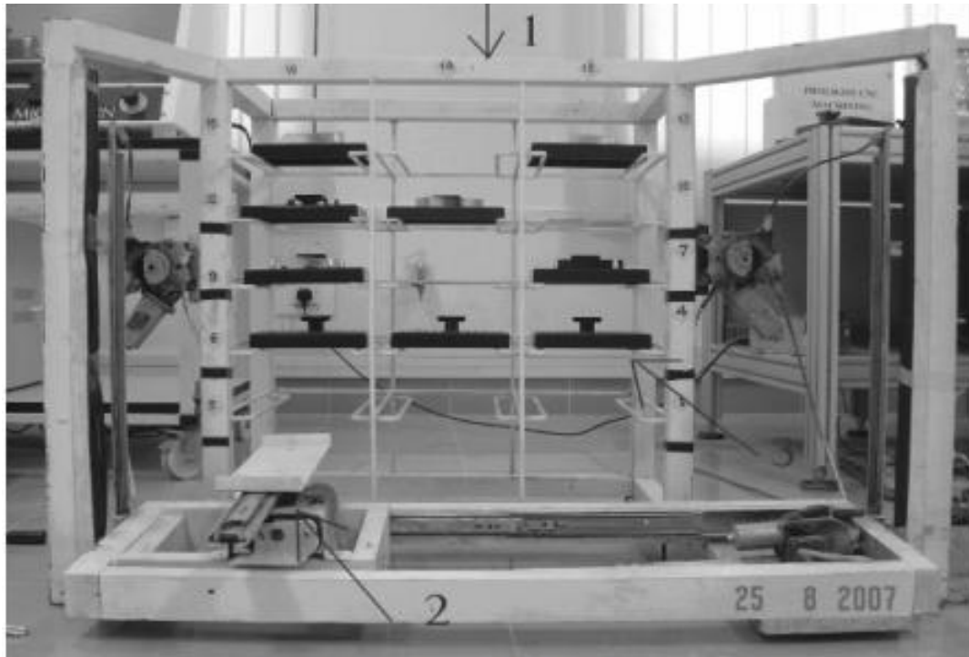
Figure 1. 5: General view of the AS/RS
