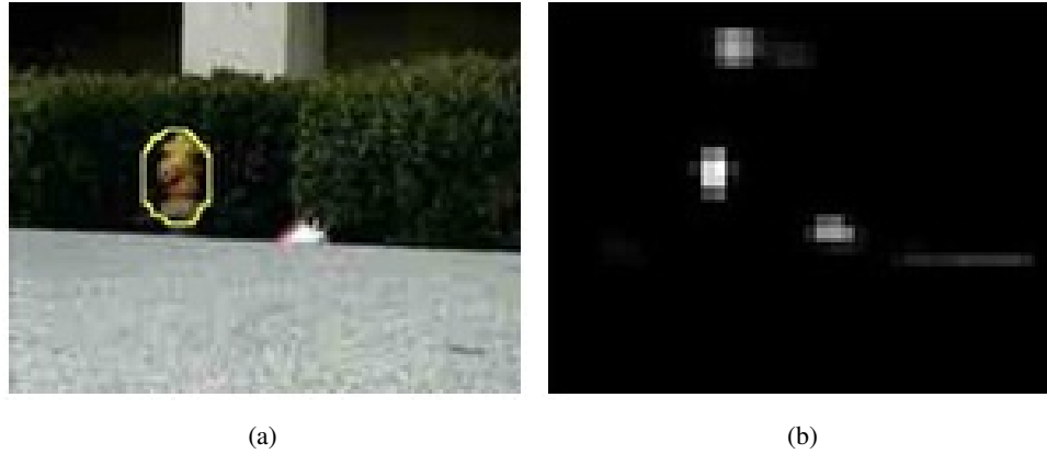
Figure 3.5: Itti-Koch Model Saliency Map (a) Input image (b) ) Itti-Koch Saliency Map of input image.
