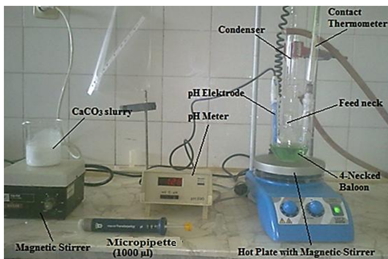
Figure 45 Experimental set-up for downstream experiments ( \text{CaCO}_3 slurry is replaceable for upcoming steps).
